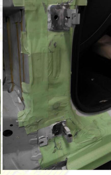
After grinding down the two-door hinge post place the new VDI hinge system against the two flat sections and mark the center of the holes. Try to get the holes as close to the center factory hinge post as possible. You will need to drill and tap one hole on at the
